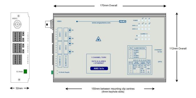
The **AMG5817** is a standalone one channel video transmit unit designed to transmit 1 video signal and transmit and receive 4 data signals plus 4 bi-directional alarms and also provides full duplex 100Base–T Ethernet connectivity over one Multimode optical fibre.
